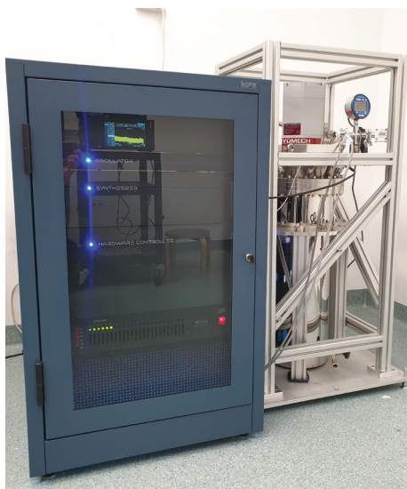
The Cryoclock is a revolutionary cryogenic sapphire oscillator, offering unmatched signal purity and stability at microwave frequencies. Credit: QuantX Labs
